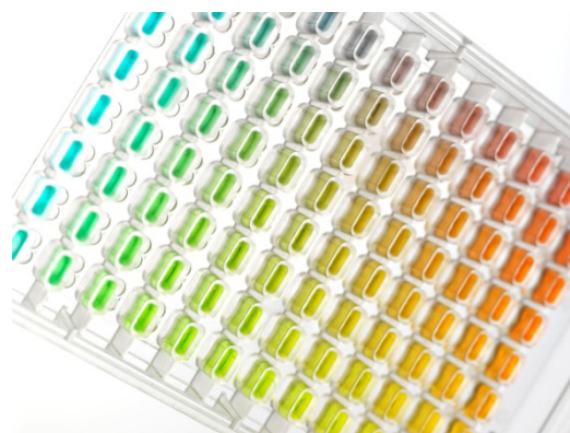
A 4 corner gradient plate for protein crystal optimisation created using TTP Labtech's dragonfly.
