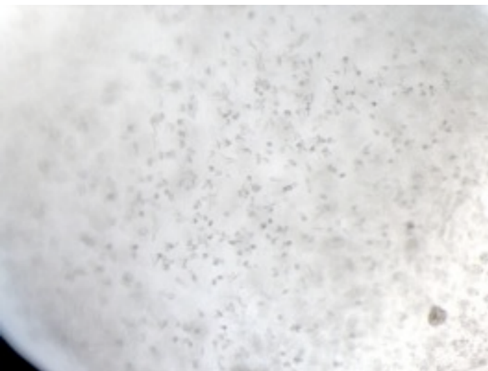
Preparative crystallization 50 mg of protein crystallized in 1 mL eppendorf tube
