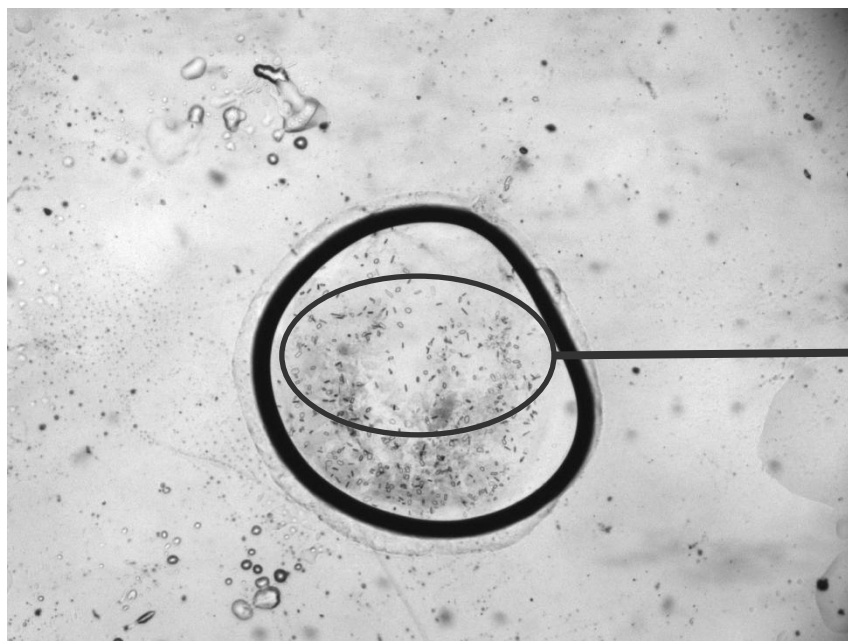
LCP drop imaged in Sandwich Plate
