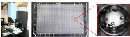
Tango LHS are used to set up 1536 unique microbatch under oil experiments for each sample in a single microassay plate (2).
