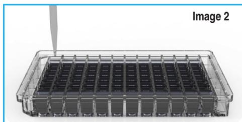
6. With the well identification correctly positioned, place the engraved UV Screen Solution Cover over the reagents for protection during dialysis.
