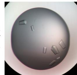
Image 1. Drop Drop experiment with 400 nl protein plus 400 nl reagent and no oil using the MRC Under Oil 96 Well Crystallization Plate.
